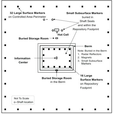
A conceptual design of WIPP's permanent marker system. DOE is evaluating other concepts. A final design will be selected prior to WIPP closure.
