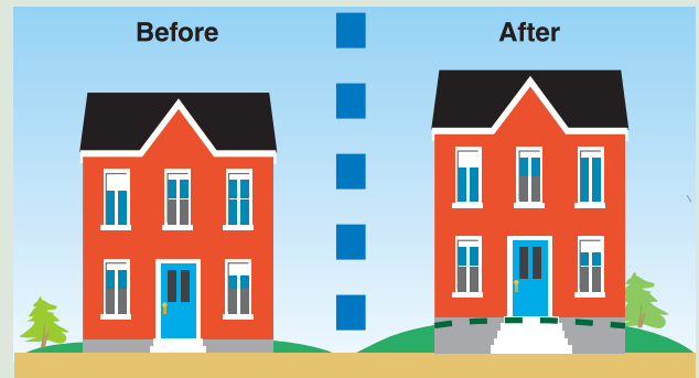
Regrading of elevated building.
